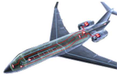
Electrical power distribution
